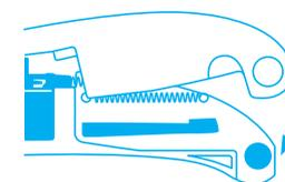
Finally, fold the **upper half of the handle back down** until it snaps into place. Please check blade retraction!
