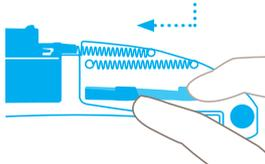
Release the blade carrier by **pressing down and pushing forward**, as indicated.
