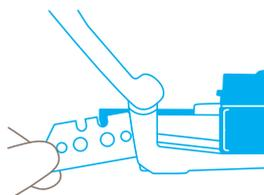
Now either **rotate or change the blade**, before pulling the blade carrier back into its original position.
