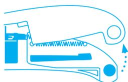
To change the blade, **press the button** at the end of the cutter and fold open the upper half of the handle.
