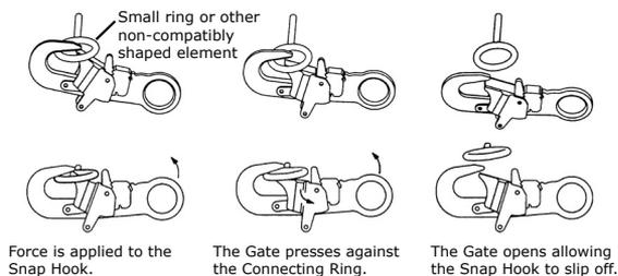
**2.4 MAKING CONNECTIONS:** Only use self-locking snap hooks and carabiners with this equipment. Only use connectors that are suitable to each application. Ensure all connections are compatible in size, shape and strength. Do not use equipment that is not compatible. Ensure all connectors are fully closed and locked.
