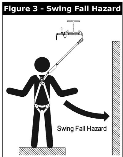
**F. FALL CLEARANCE:** There must be sufficient clearance below the user to arrest a fall before the user strikes the ground or other obstruction. The clearance required is dependent on the following factors:
