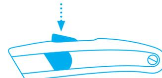
Now **rotate or change the blade** and carefully release hold of the slider. Close the rocking device.
